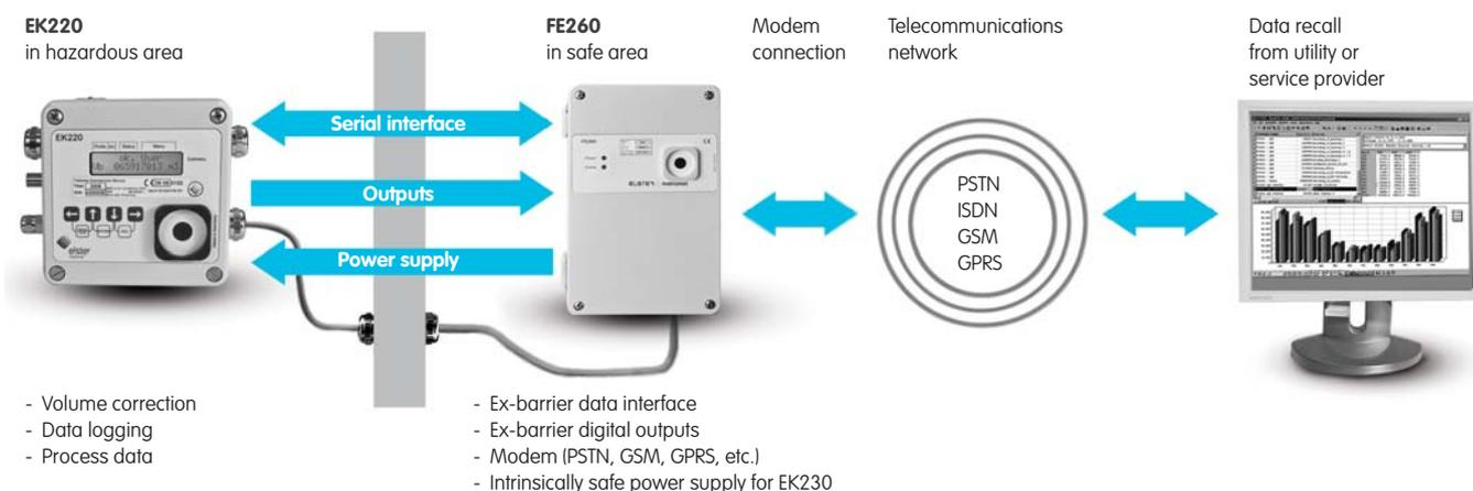
The Ex-barrier of the serial interface and the pulse outputs of the volume corrector is provided by function extension unit
